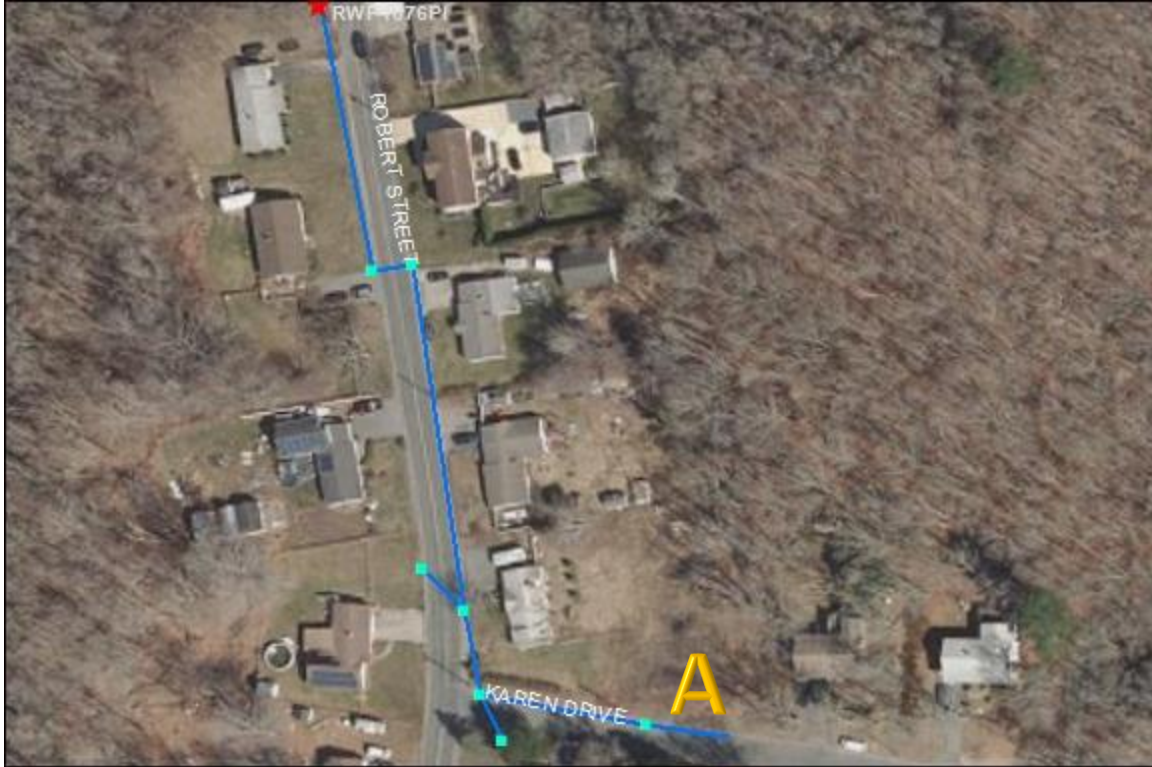
RWP1076PI-Robert Street: No issues found. A twelve-inch metal pipe was observed entering the catchbasin at point A. Its origin is unknown. Further investigation is suggested. Outfall was inventoried.
