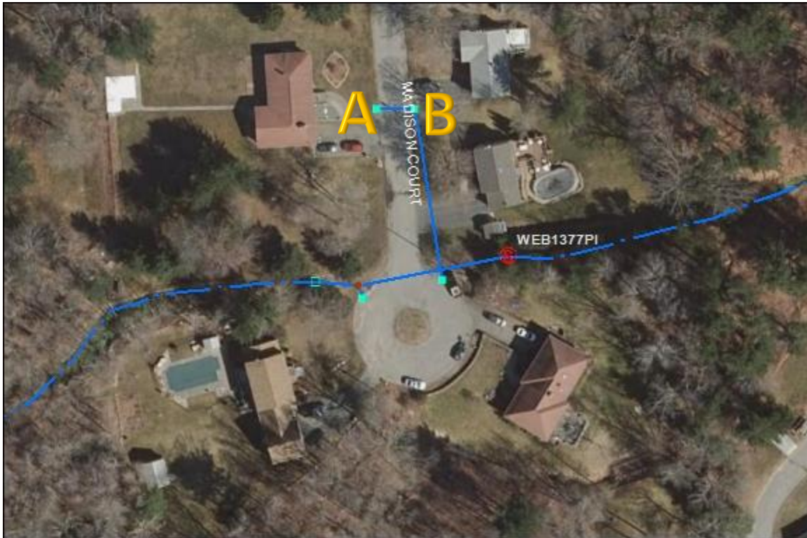
RWP1076PI-Robert Street: No issues found. A twelve-inch metal pipe was observed entering the catchbasin at point A. Its origin is unknown. Further investigation is suggested. Outfall was inventoried.
