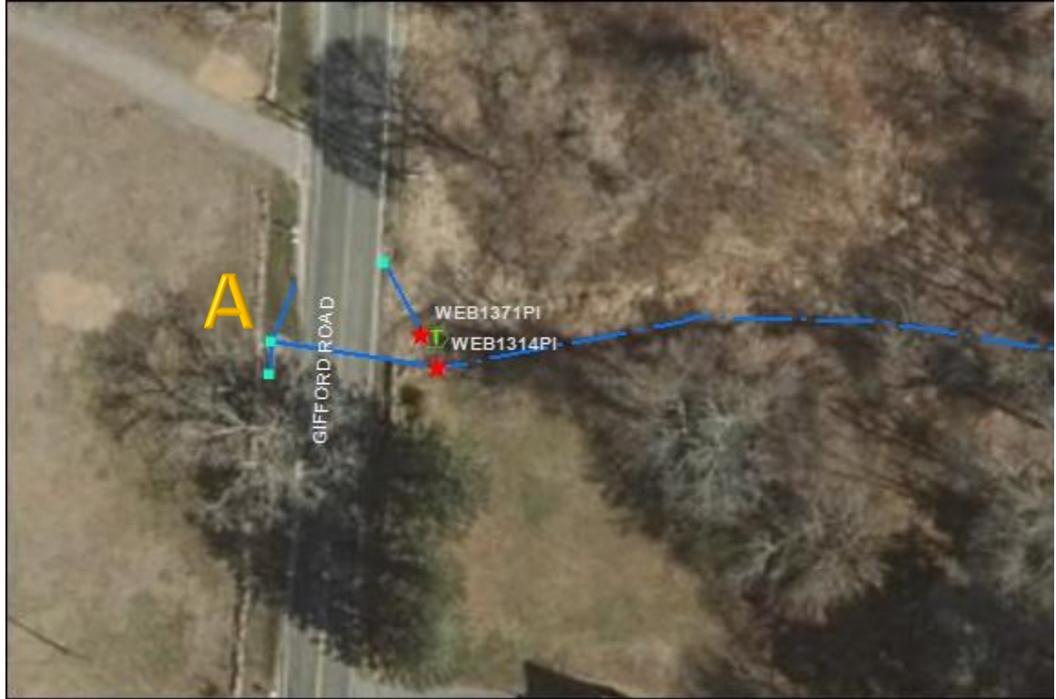
WEB1371PI and WEB1314PI- Gifford Road: No significant issues found. At point A, a pipe enters the catchbasin its origin is unknown. Further investigation is recommended.
