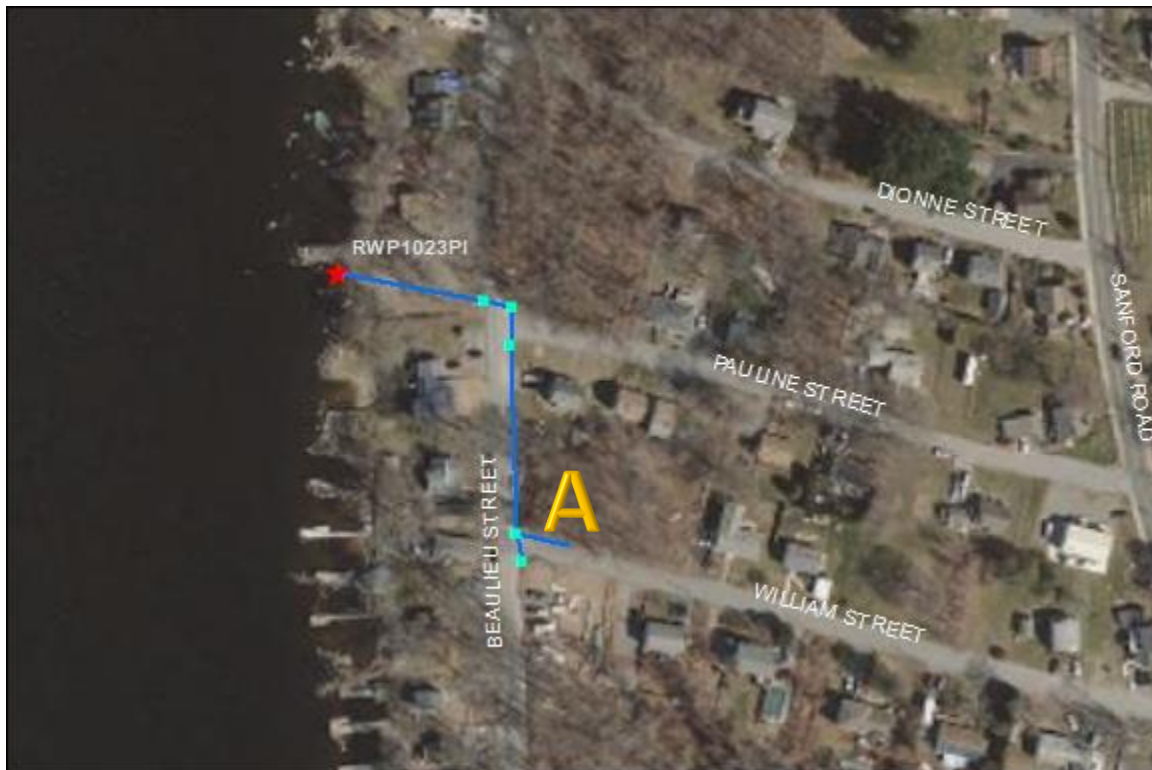
RWP1023PI- Beaulieu Street: No issues found. At point A, a 15" metal pipe enters the catchbasin. Its origin is unknown. Further investigation is suggested.
