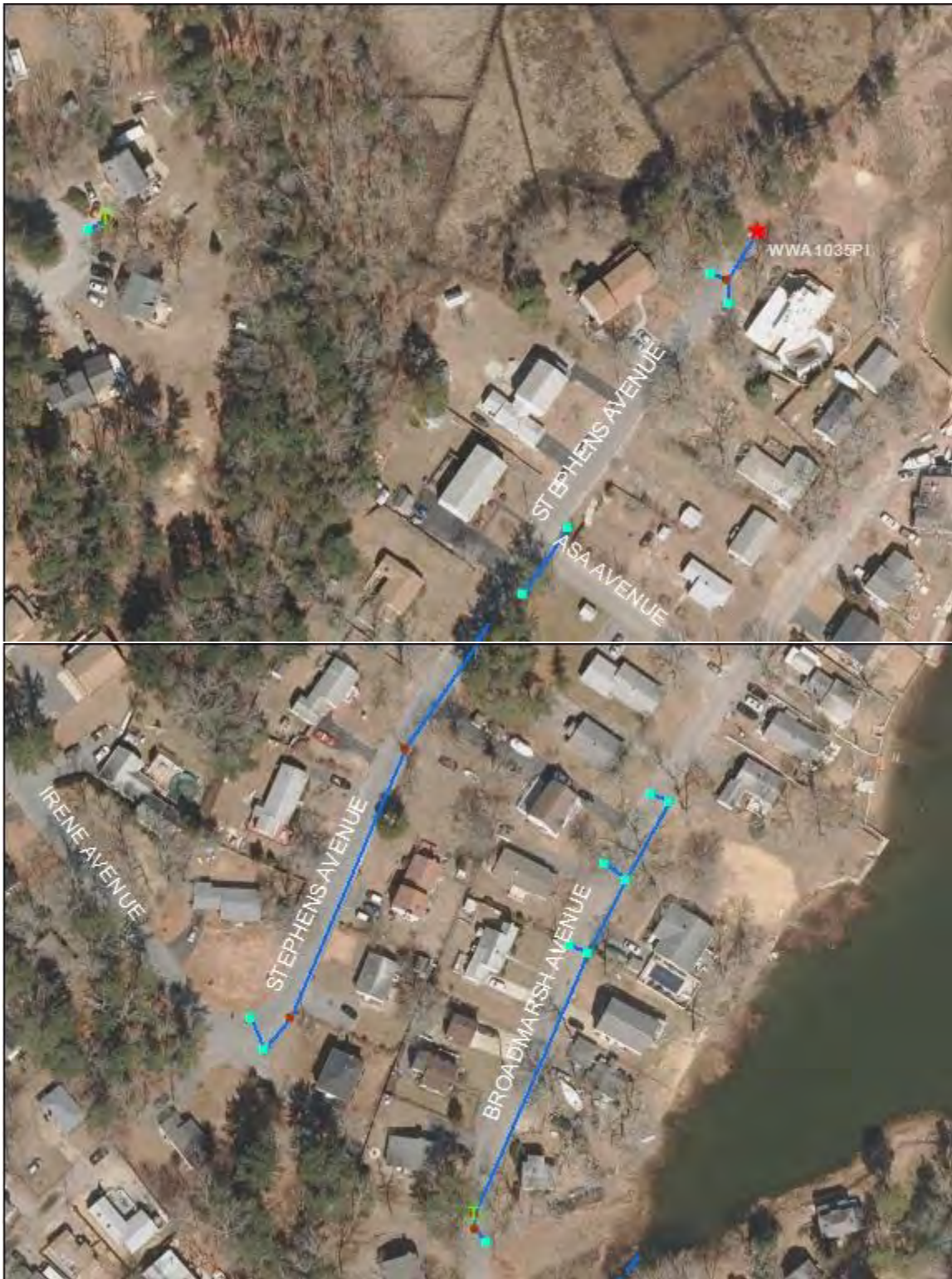
WWA1035pi- Stephens Avenue and Broadmarsh Avenue: No significant issues found. All catchbasins on Broadmarsh Avenue have 12" metal pipes that are clogged. Residents informed that it floods in this area often. Further maintenance is strongly suggested.
