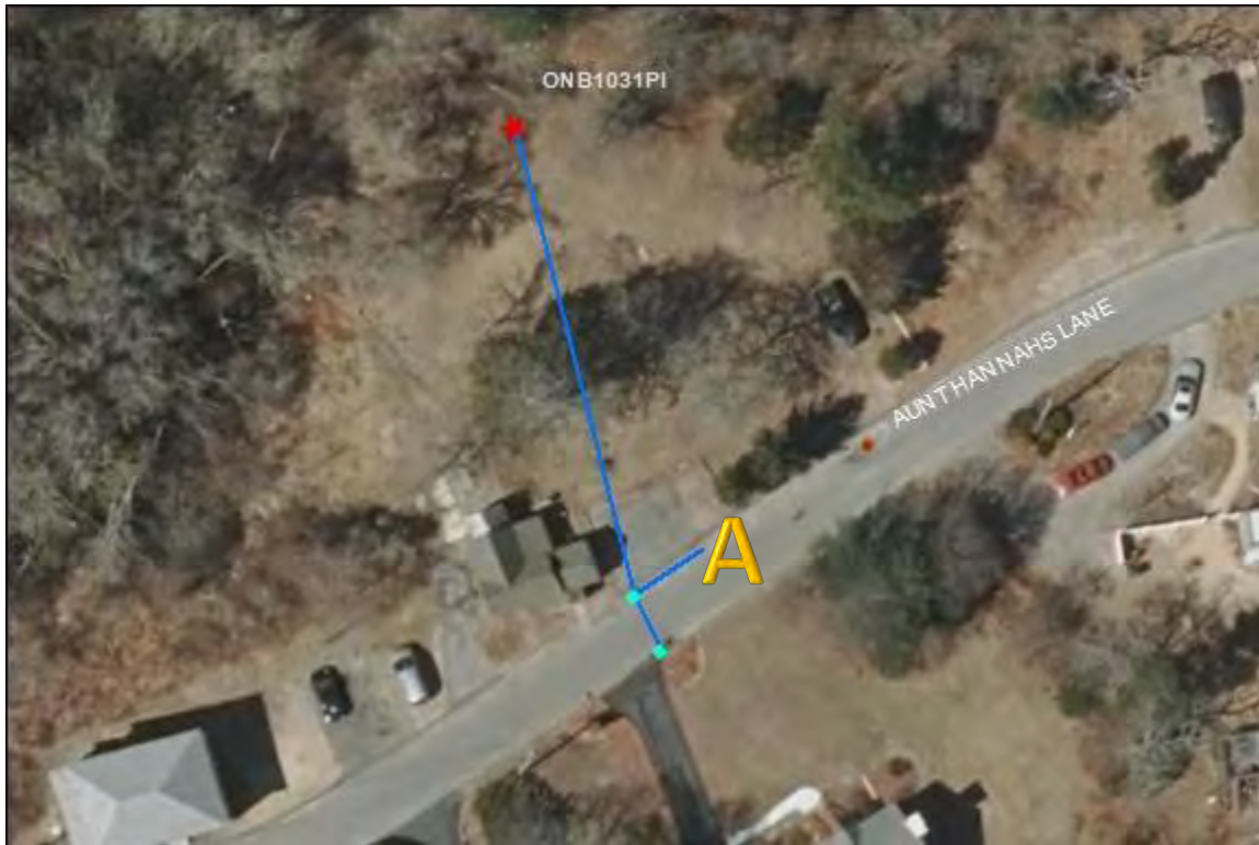
ONB1031PI- Aunt Hannahs Lane: No issues found. At point A here is an incoming pipe. Its origin is unknown. Further inspection is suggested.
