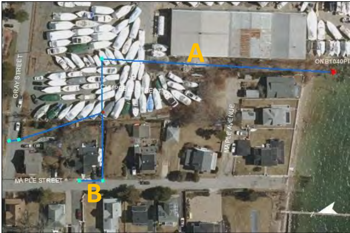
ONB1040PI- Gray Street and Maple Street: Pipe shown at point A is extremely blocked, most likely collapsed. Flooding occurs in the boat yard and at the Northwest catch basins shown at point B. Blockage of pipe needs to be repaired.
