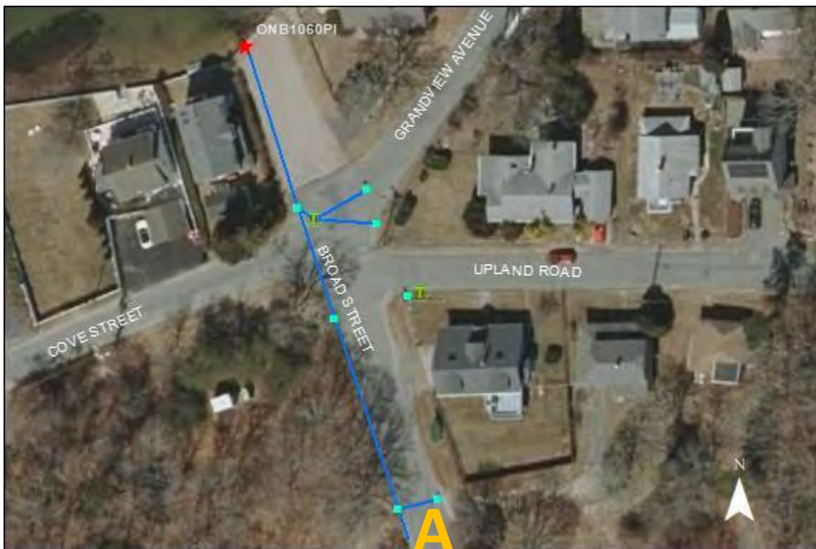
ONB1060PI- Grandview Avenue at Broad Street: No issues found. At point A, a pipe enters the catch basin. Its origin is unknown. Further investigation is recommended.
