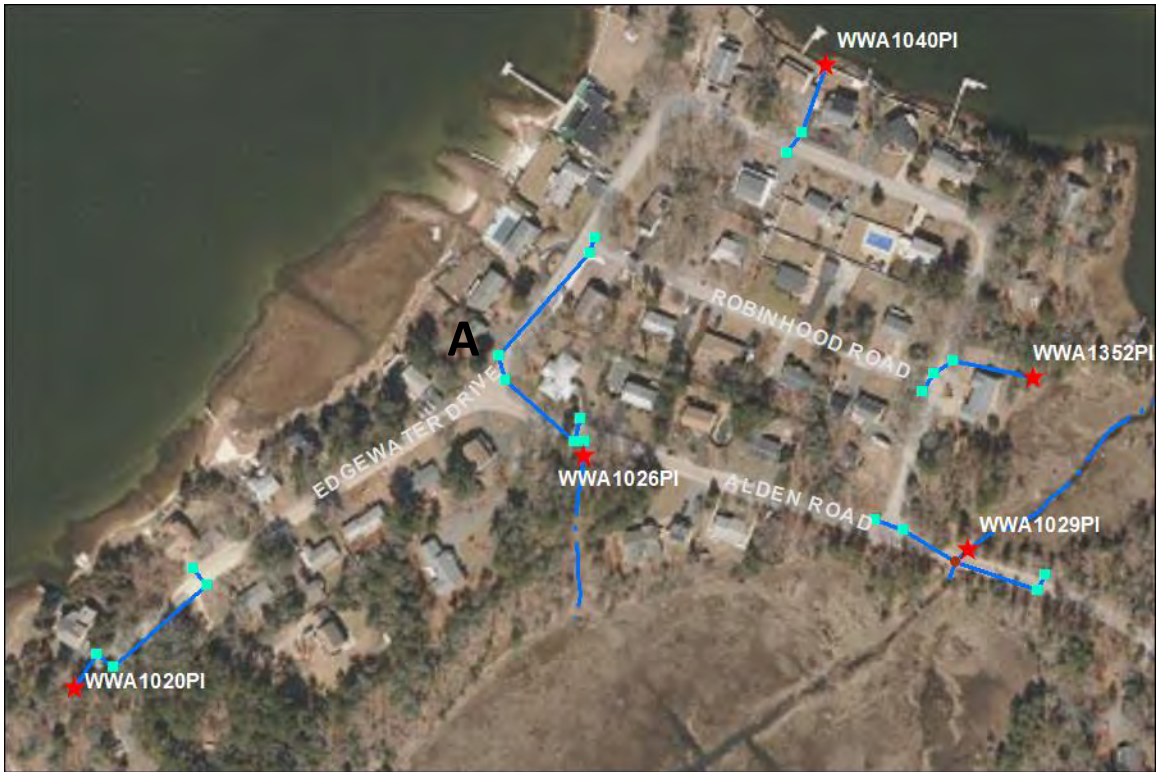
WWA1020PI, WWA1026PI, WWA1040PI, WWA1352PI, and WWA1029PI – Edgewater Drive and Alden Road: No issues found; at location A homeowner stacked bricks on catch basin preventing access.
