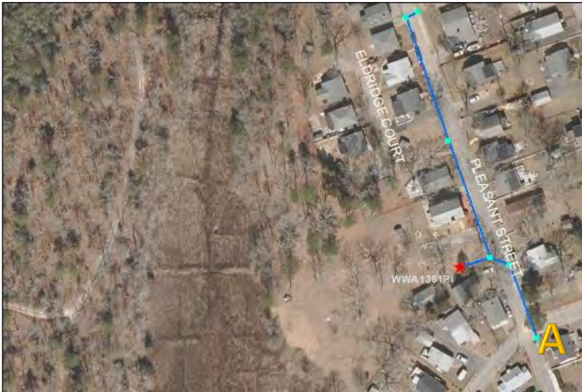
WWA1361PI- Pleasant Street: No significant issues found. At point A the catchbasin had a lot of trash and leaf debris. Further maintenance is suggested.
