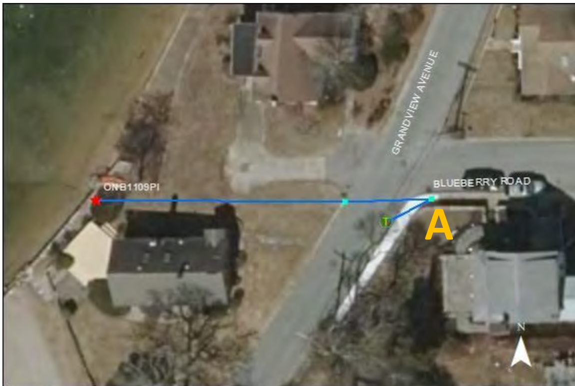
ONB1109PI- Grandview Avenue at Blueberry Road: Manhole at point A is full of sand. Catchment is in need of cleaning and reinspection. Further action is recommended.
