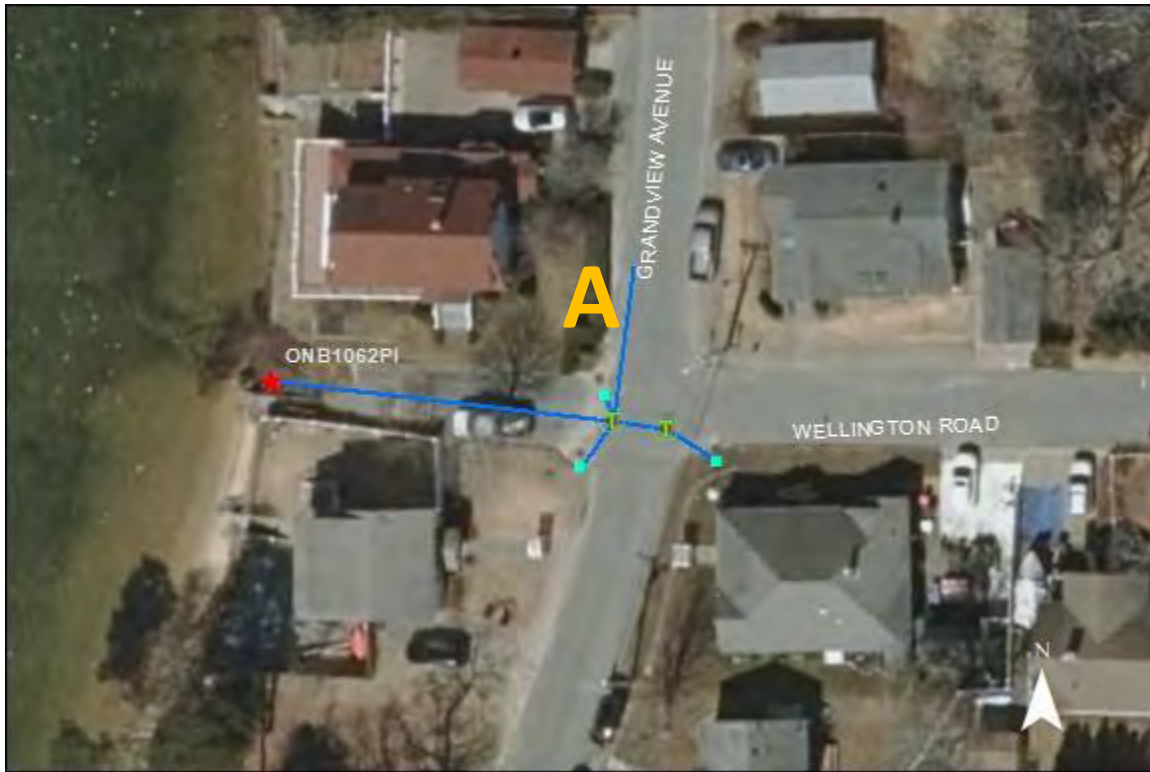
ONB1062PI- Grandview Avenue at Wellington Road: No issues found. At point A, a pipe enters the manhole; its origin is unknown. Further investigation is recommended.
