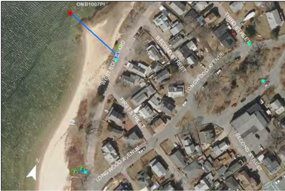
ONB1007PI- West Boulevard: No issues found. Basins on Longwood at Third Street are stand alone basins.
