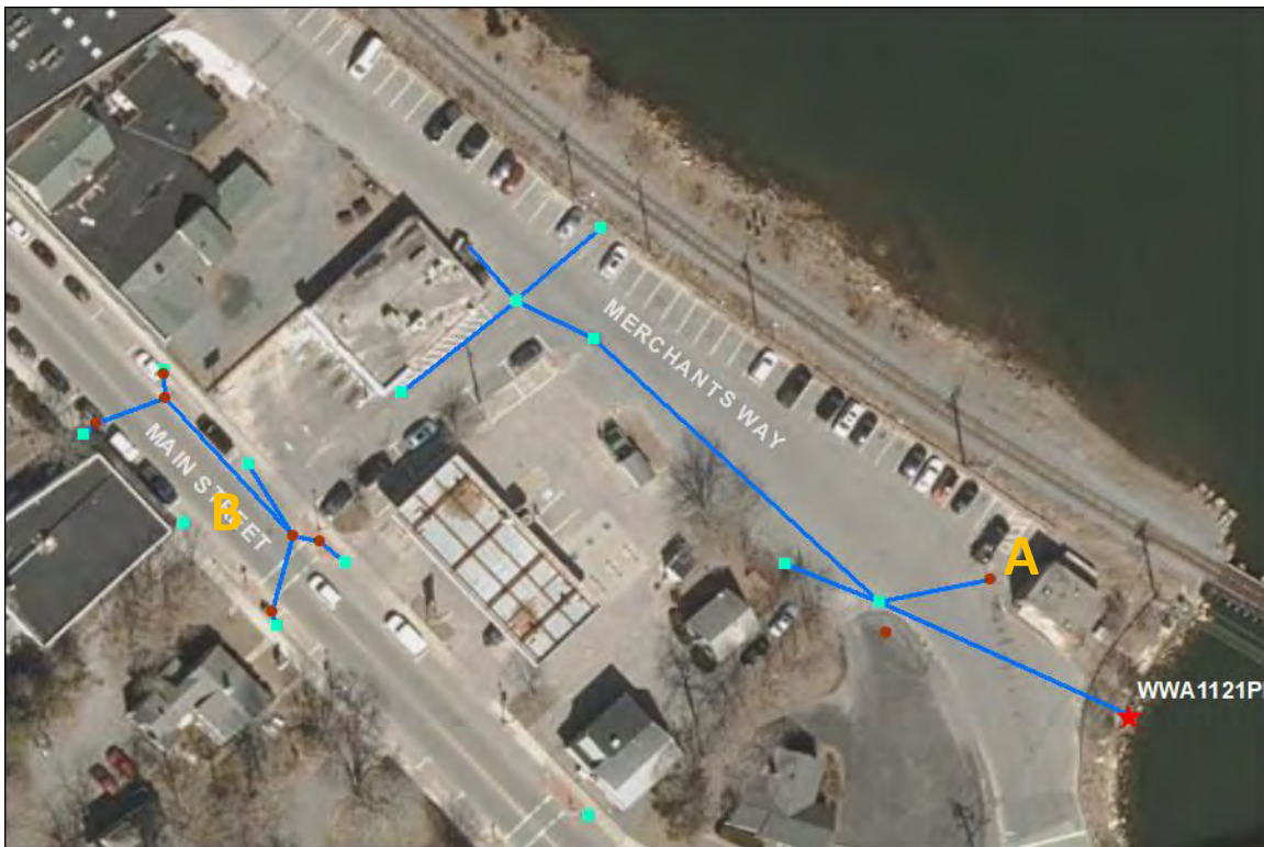
WWA1121PI – Merchants Way: No issues found; manhole at location A appears to be an unused interface with the sewage pump station; area at location B connectivity to network not determined; requires follow-up.
