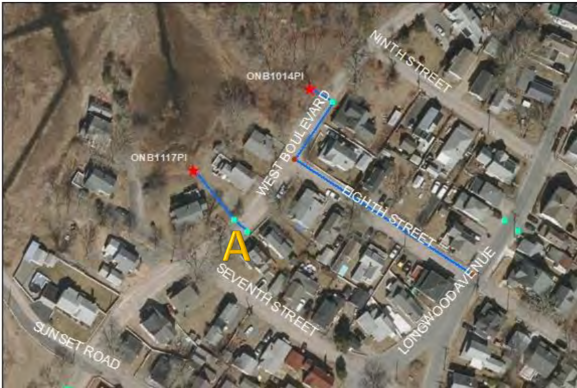
ONB1117PI and ONB1014PI- West Boulevard: No significant issues found. At point A the catchbasins flood. There appears to be a lot of blockages in the pipes at that location. Further maintenance is suggested.
