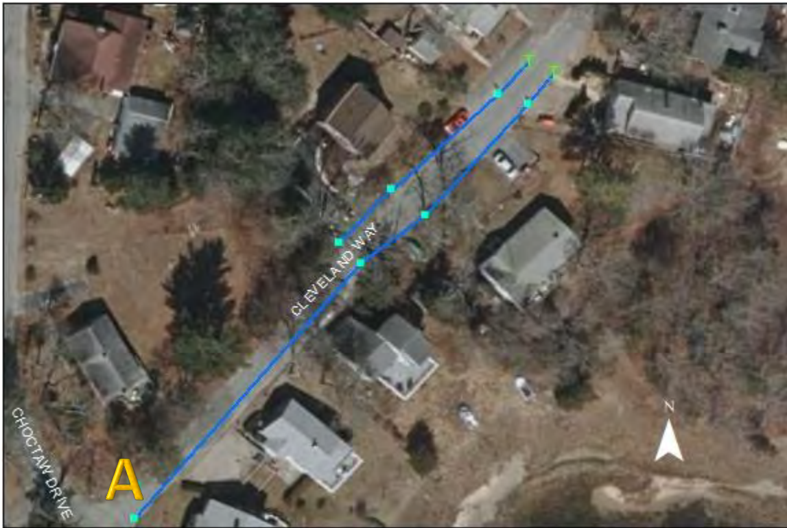
Cleveland Way: At point A the catchbasin is full of water. All other basins were dry. Highly likely the pipe exiting the basin is clogged. Neighbors reported major flooding during rain events. Maintenance is recommended.
