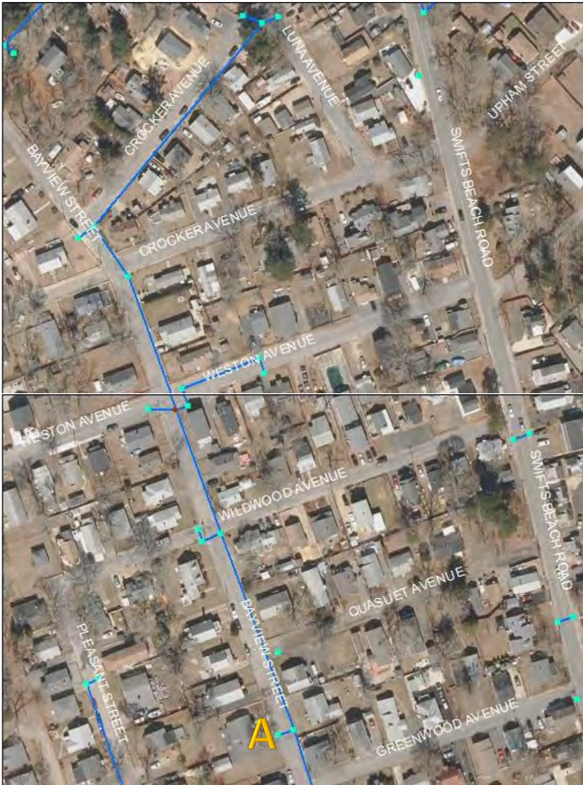
Bayview Street: No significant issues found. At point A the catchbasin has begun to sink. Preventative maintenance is suggested.
