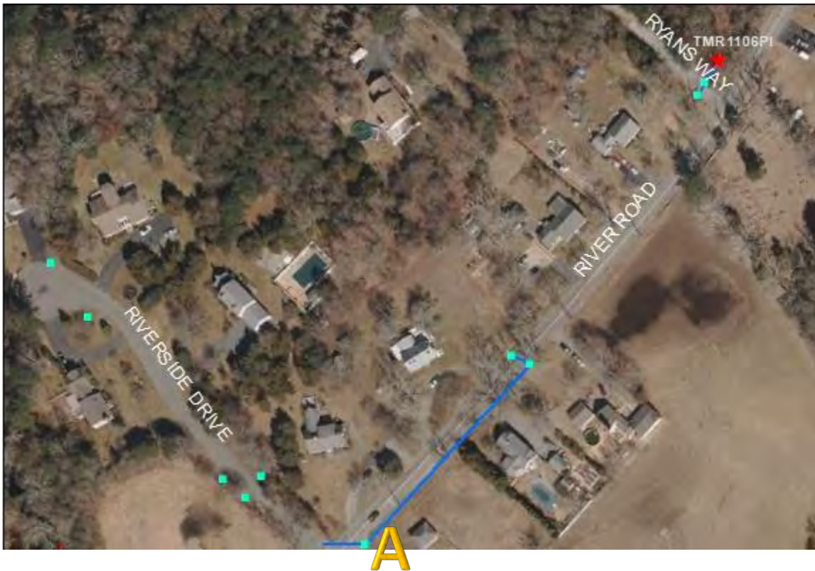
TMR1106PI- Ryans Way: No issues found. Riverside Drive: Catchbasins are infiltration basins. No issues found. River Road: Catchbasin at point A has a blocked pipe exiting it. Drainage outfall could not be determined due to this. Maintenance and reinspection are recommended.
