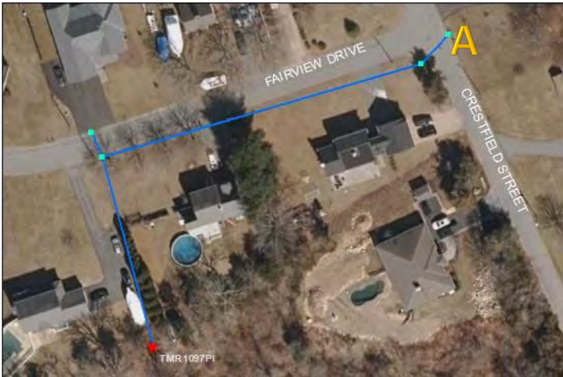
TMR1097PI- Fairview Drive and Crestfield Street: At point A there is an incredible amount of dog waste bags, roughly 50. Cleaning of the catchbasin and community outreach is strongly recommended.
