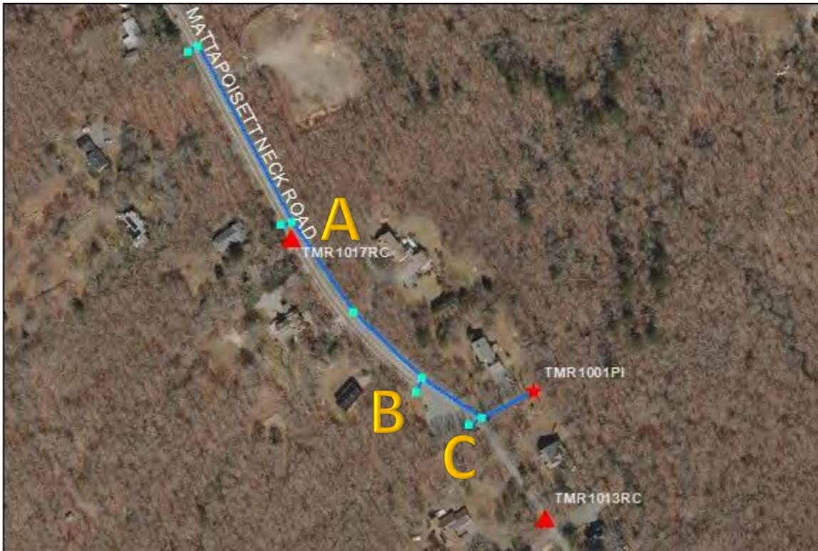
TMR1001PI, TMR1017RC, and TMR1013RC- Mattapoissett Neck Road: No significant issues found. Catchbasins at point A, B, and C have begun to sink. Preventative maintenance is suggested.
