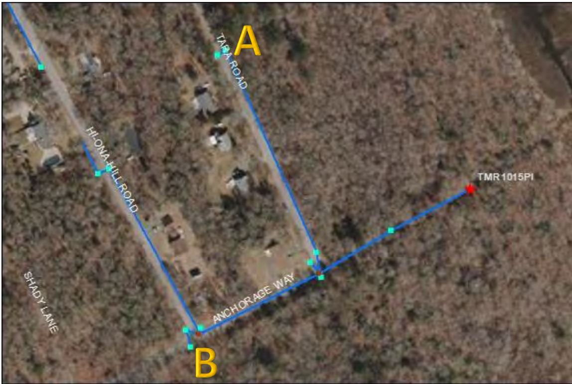
TMR1015PI- Tara Road, Hi-Ona-Hill Road, and Anchorage Way: No significant issues found. At point A and B, the catchbasins are both beginning to sink. Preventative measures are recommended.
