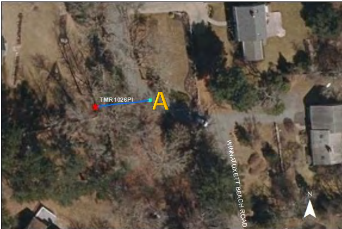
TMR1026PI- Winnatuxett Beach Road: At point A the catchbasin is sinking. Further attention is needed.
