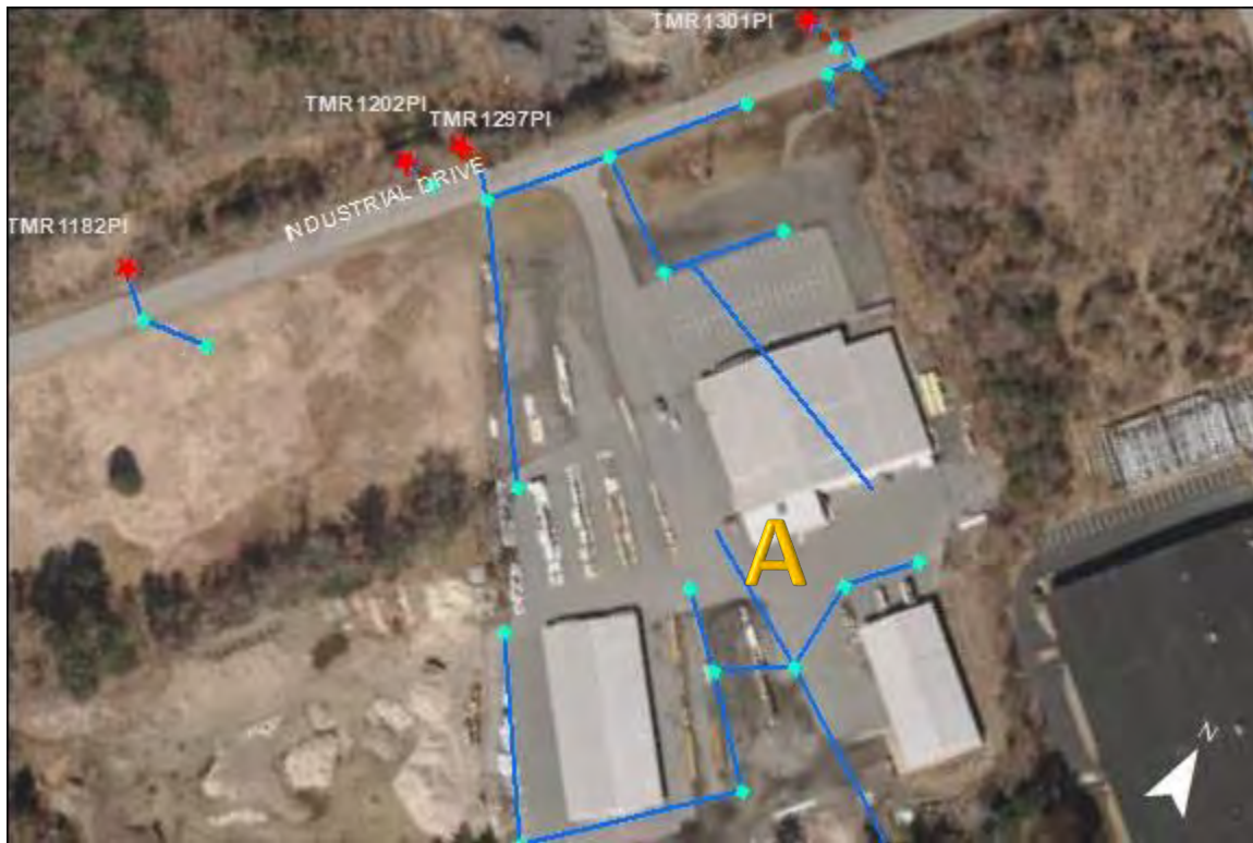
TMR1182PI TMR1202PI, TMR1297PI, and TMR1301PI- Industrial Drive: No issues found. At point A there is a steady flow of water flowing through the pipe. Its destination is unknown. It did not connect to stormwater infrastructure on Industrial Drive. Further investigation is suggested.
