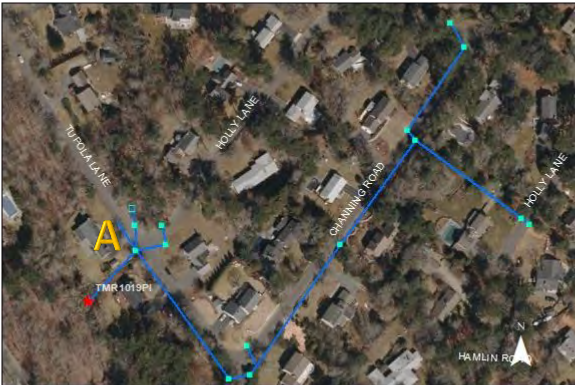
TMR1019PI- Tupola Lane and Channing Road: No issues found. At point A an 8" metal pipe enters the catchbasin. Its origin is unknown. Further investigation is suggested.
