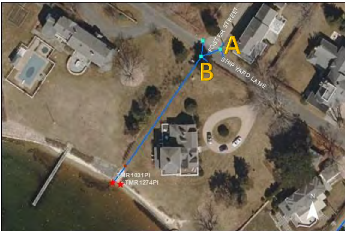
TMR1031PI and TMR1274PI- Ship Yard Lane: No issues found. Multiple pipes shown at point A and B enter the catchbasins. Their origins are unknown. Further investigation is suggested.
