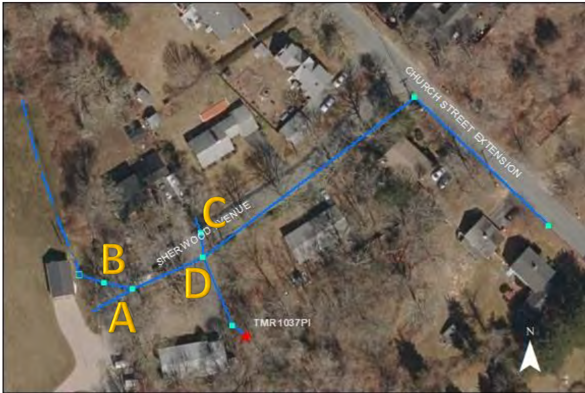
TMR1037PI- Sherwood Avenue: At point A, a 12" PVC pipe enters the catchbasin. Its origin is unknown. Further investigation is suggested. At points B, C, and D the catchbasins have begun to sink. Preventative measures are strongly recommended.
