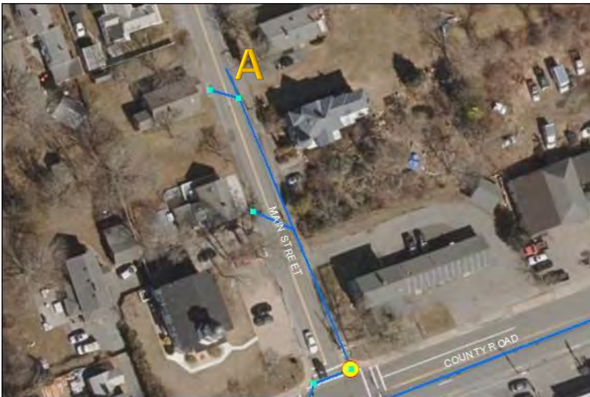
Main Street N of County Road: No issues found. Interconnection between Mattapoisett's stormwater system and the state's stormwater system. At point A, a 12" metal pipe enters the catchbasin. Its origin is unknown. Further investigation is recommended.
