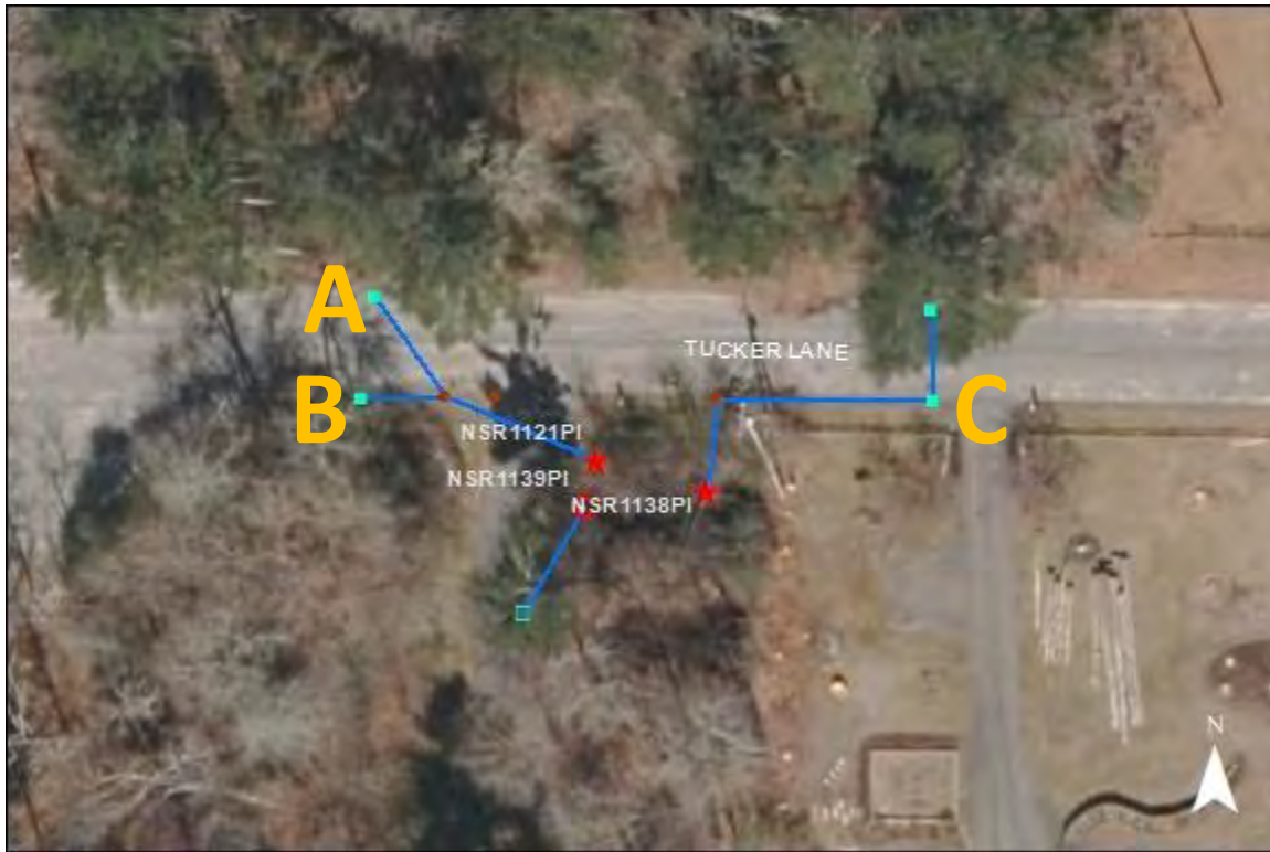
NSR1121PI, NSR1139PI, and NSR1138PI- Tucker Lane: Catchbasins at A, B, and C have all begun to sink. Preventative maintenance is recommended.
