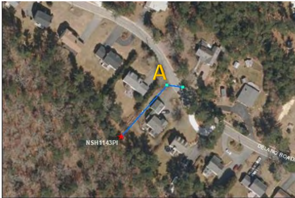
NSH1143PI- Delano Road: No significant issues found. At point A the road floods during rain events. There is a small 4" HDPE pipe located above ground to help relieve this issue. However, it does not extend far enough to drain the water retention in front of house #529. Further remediation is recommended.
