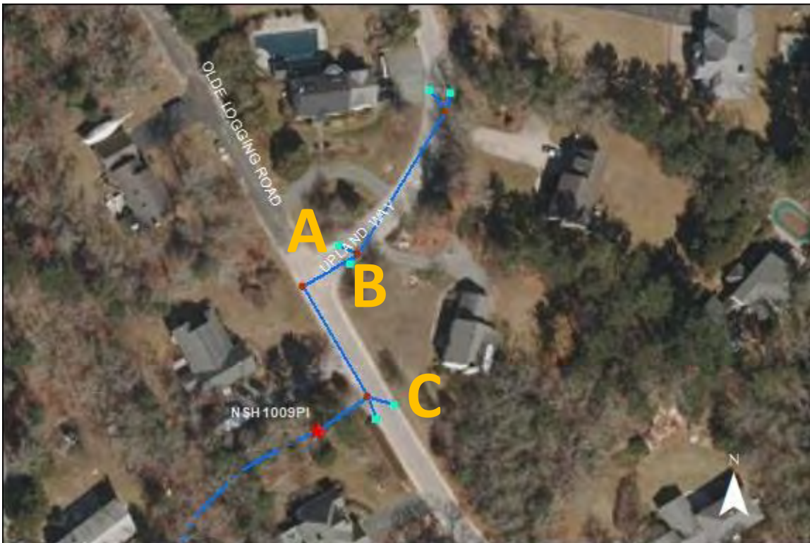
NSH1009PI- Upland Way and Olde Logging Road: At point A, B, and C, the catchbasins are beginning to sink and the frames are beginning to chip. Preventative maintenance is recommended.
