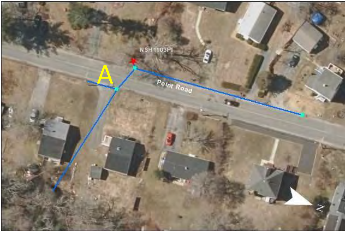
NSH1103PI- Point Road: No issues found. Pipe enters catchbasin at point A. Origin of pipe unknown.
