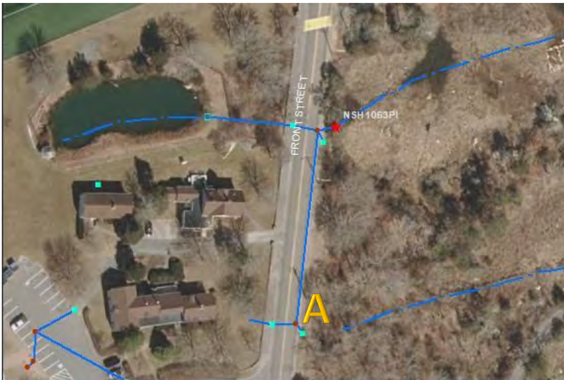
NSH1063PI- Front Street: No significant issues found. The manhole at point A was packed with dirt and had significant root growth. The Town cleaned it out and the connection between manholes was confirmed. It has previously flooded in this area. Further maintenance within the pipes may still be needed to avoid this.
