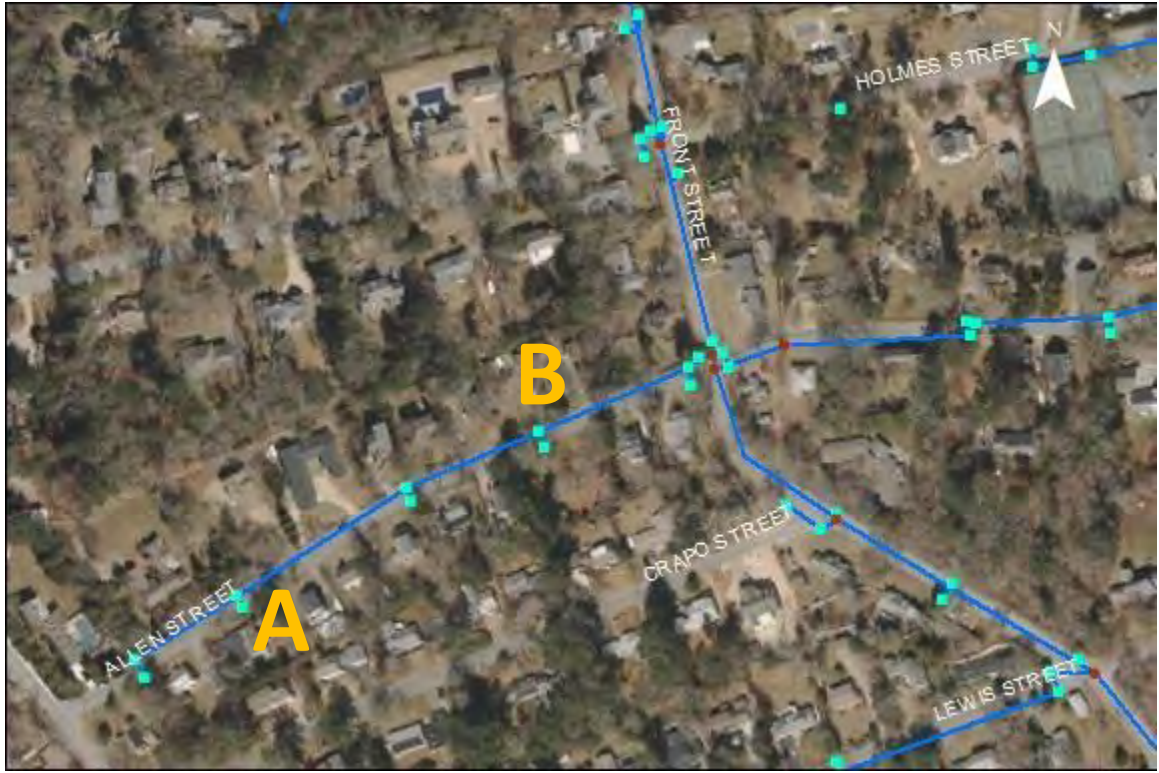
NSH1019PI (2/3)- Front Street: At point A and B the catchbasins have begun to sink. Both are in need of repair. Preventative maintenance is recommended.
