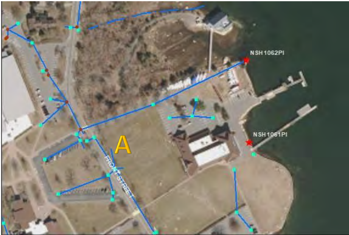
NSH1062PI and NSH1061PI – Front Street: No issues found. The catchbasins at the sailing center do not appear to connect to the Town’s network. At point A, a pipe exits the catchbasin in the direction of a wetland. The wetland fills with water during rain events. Extremely likely there is an outfall buried there that is fully functioning. However, it could not be confirmed.
