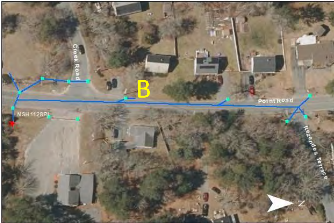
NSH1128PI-Point Road and Creek Road: No issues found. At point B a 12" pipe enters the catchbasin. Its origin is unknown.
