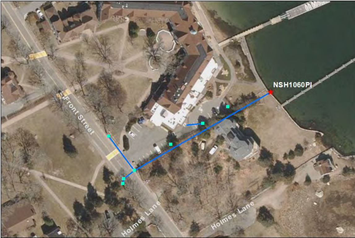
NSH1060PI – Front Street: No issues found. The catch basins in the dining hall parking lot do not connect to this network. They appear to connect to the grease trap which drains to the sewer system causing inflow.
