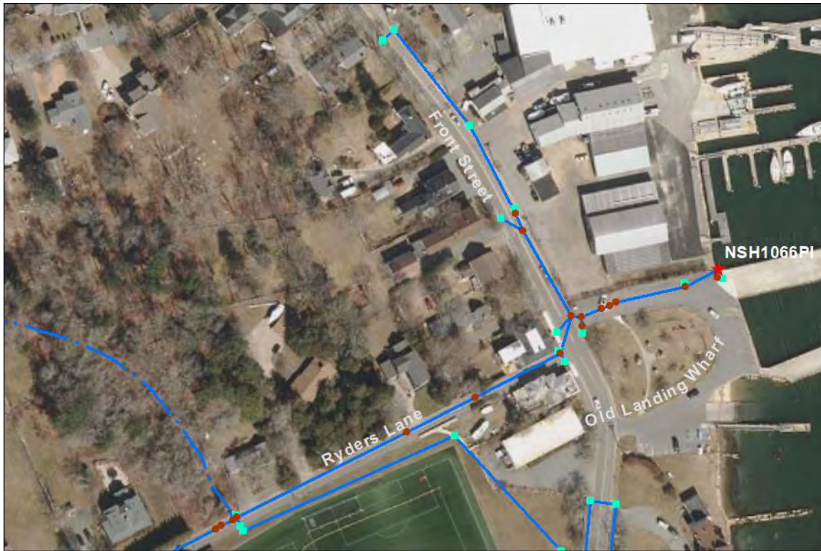
NSH1066PI (1/2) – Front Street and Ryders Lane: No issues found. This system was installed in 2013 to re-route the stream North of Ryders Lane from traversing the ball field and directs it to a treatment system at Old Landing Wharf.
