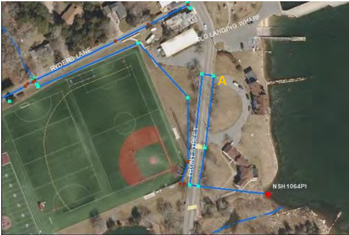
NSH1064PI- Front Street: No issues found. The NSH1064PI network used to traverse the ball field but has been rerouted around the field. At location A the catch basin is covered with a silt fence.
