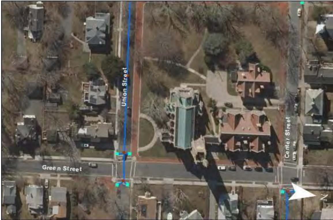
FIH1106PI- Union Street: At point A, a pipe enters the catchbasin. The origin of the pipe is unknown. At the corner of William Street and Union Street, at point B, there is a connection between the stormwater system and the sewer system. This needs immediate attention. Since the first version of this report the connection has been blocked. Is now in good order.
