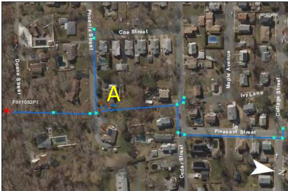
FIH1053PI- Phoenix Street, Cedar Street, and Pleasant Street: No issues found. At point A there is a very old manhole with a pipe entering and exiting. The origin and destination of these pipes is unknown.
