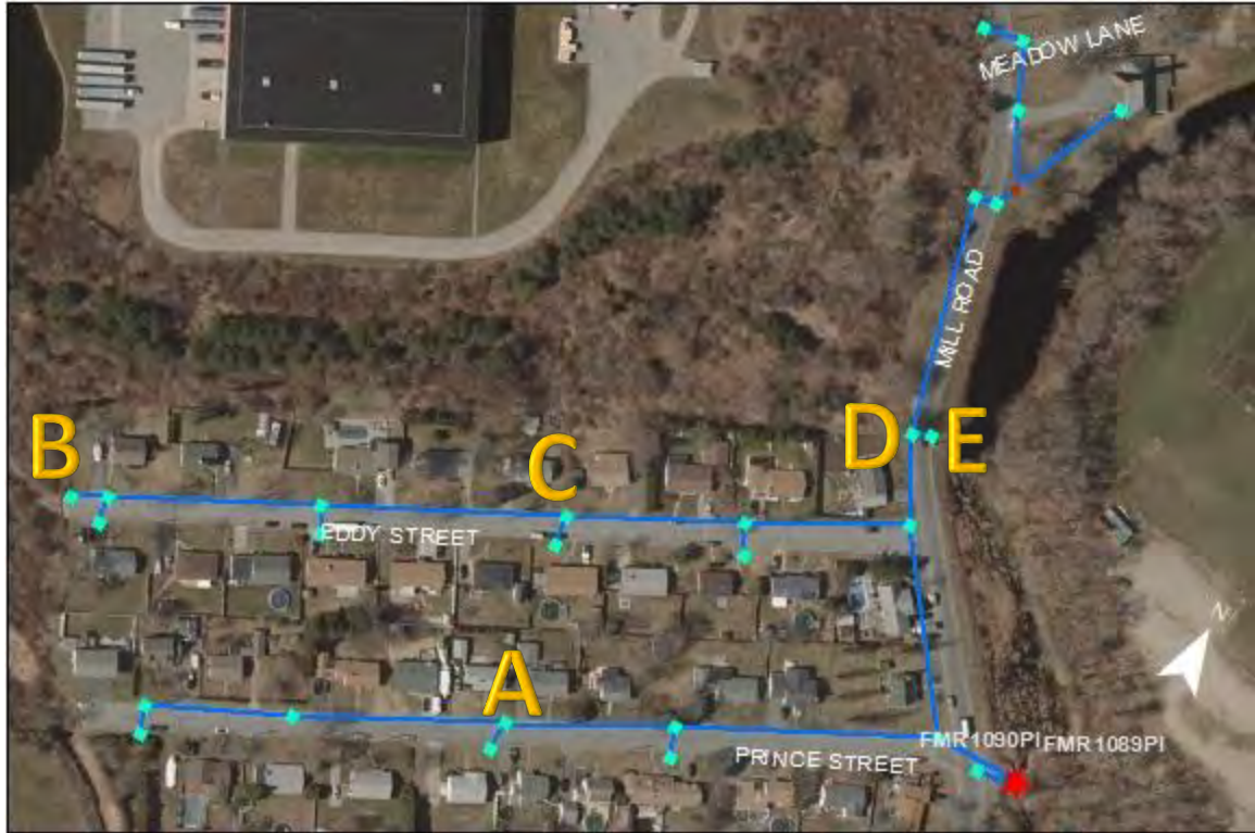
FMR1090PI and FMR1089PI- Mill Road, Eddy Street, and Prince Street: The catchbasins at A, B, C, D, and E are sinking. Further maintenance is recommended.
