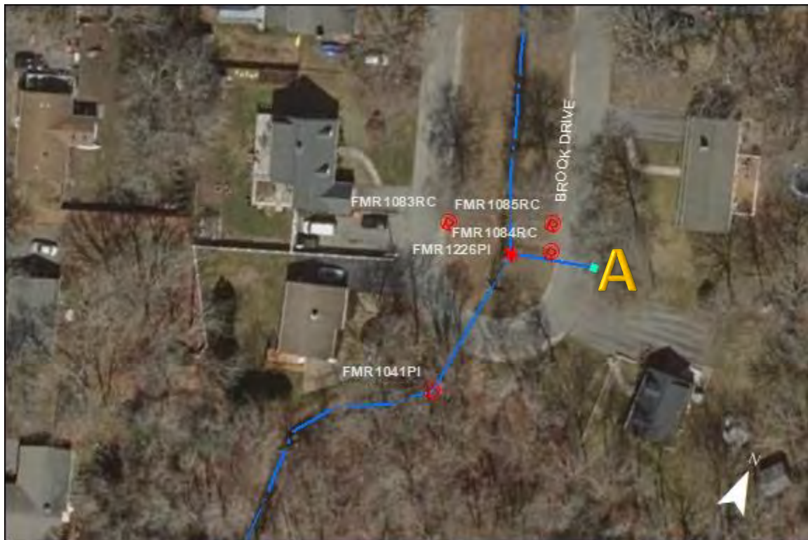
FMR1083RC, FMR1085RC, FMR1084RC, FMR1226PI, and FMR1041PI- Brook Drive: At point A the catchbasin is inking. Further maintenance is recommended.
