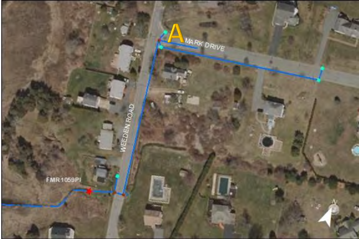
FMR1059PI- Weeden Road and Mark Drive: No significant issues found. At point A, a 12" concrete pipe enters the manhole. Its origin is unknown. Further investigation is recommended.
