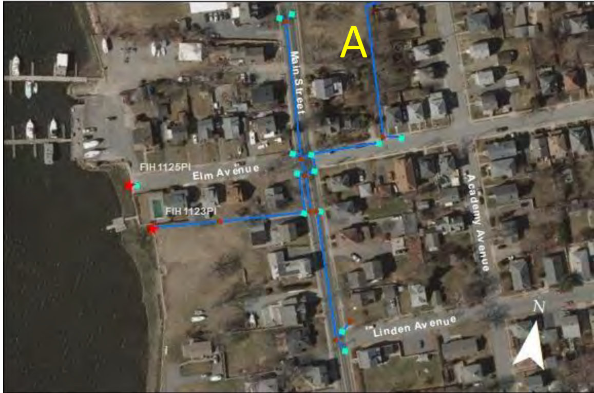
FIH1123PI- Main Street: No issues found. Note that this catchment is connected to catchment FIH114PI by way of an underground culvert illustrated at point A.
