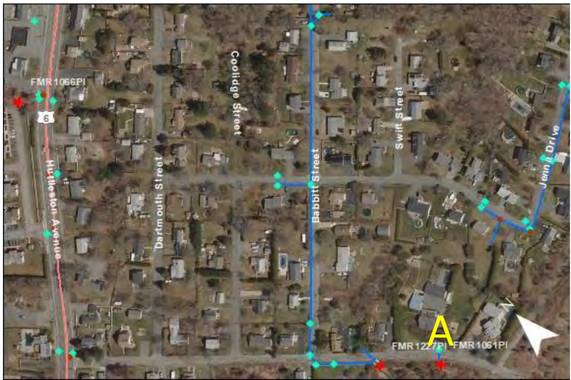
FMR1060PI and FMR1227PI- Evergreen Street and Babbitt Street: No issues found. Multiple structures have incoming pipes with unknow origins. Further investigation is recommended.
