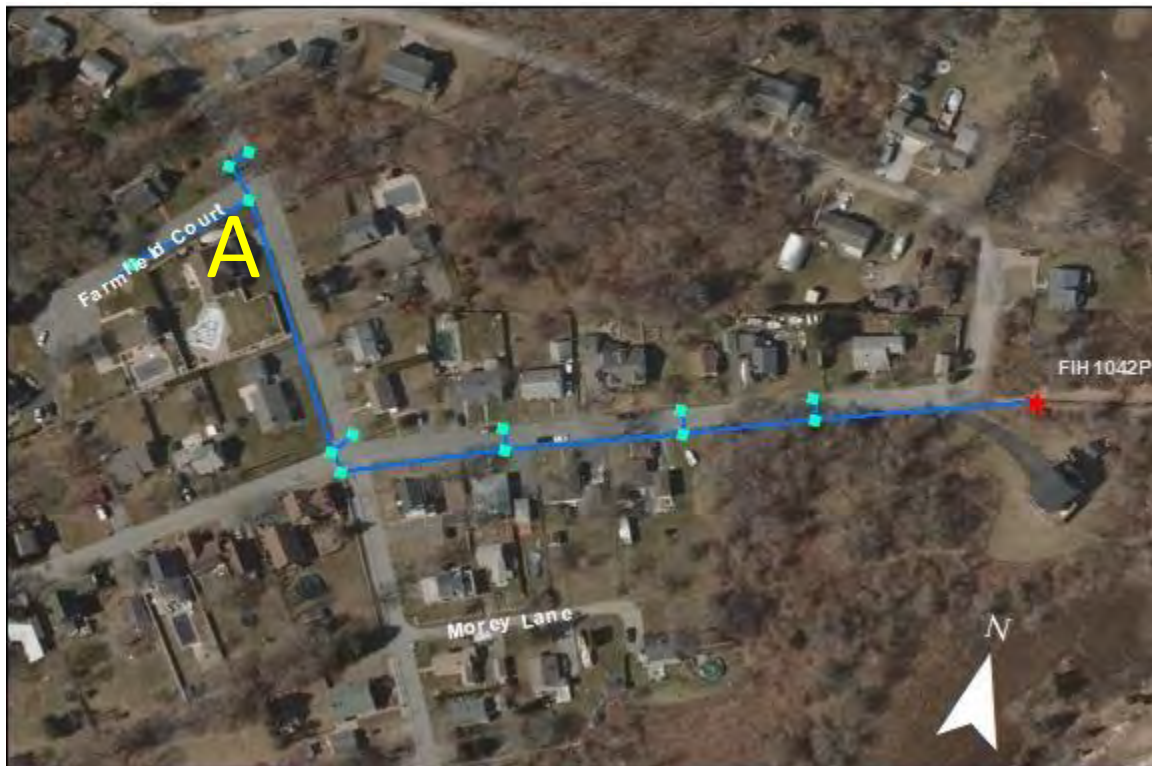
FIH1042PI- Cedar Street and Farmfield Court: No issues found. At point A, a pipe enters the catchbasin. Its origin is unknown, but it is likely it is remnant from a structure that is no longer in use.
