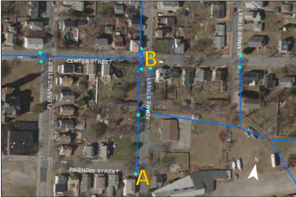
(1/2) FIH1051PI- Adams Street: At point A and B the structures were full of water. Likely that there is a blockage in each one. Friendly Street floods during rain events. Further maintenance is highly suggested.
