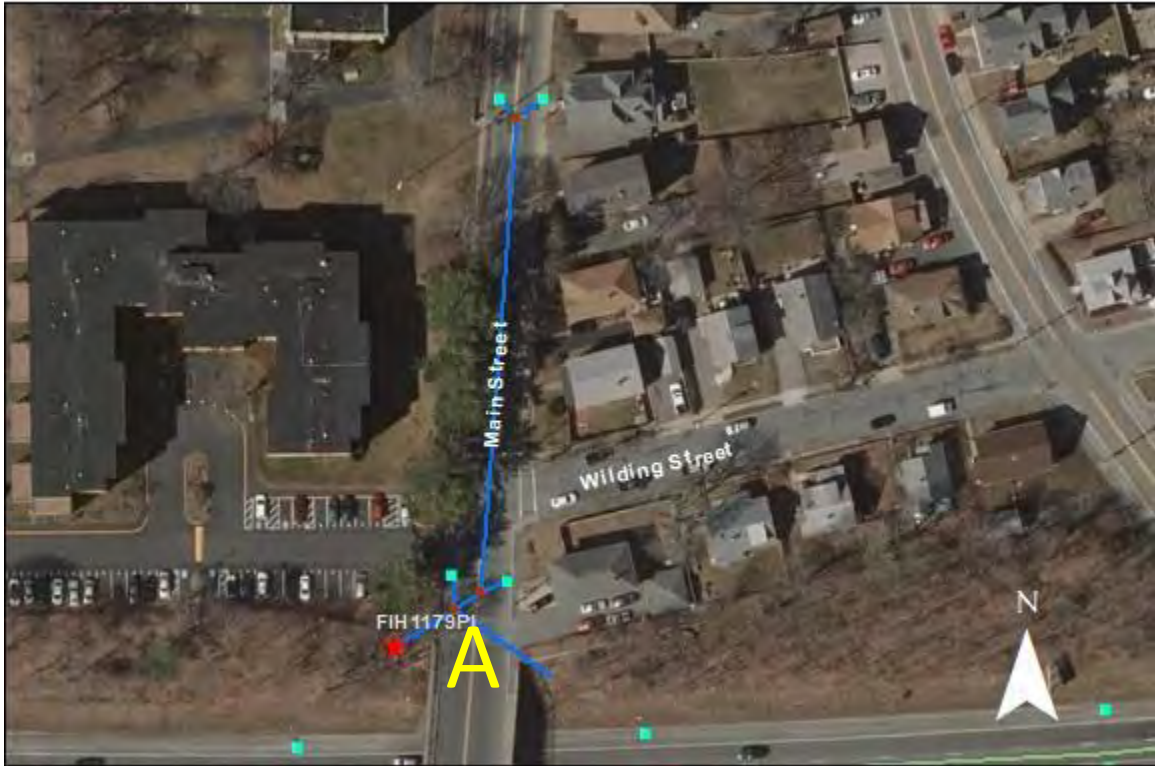
FIH1179PI- Main Street: No issues found. The manhole at point A has an incoming pipe with an unknown destination. Further investigation is suggested.
