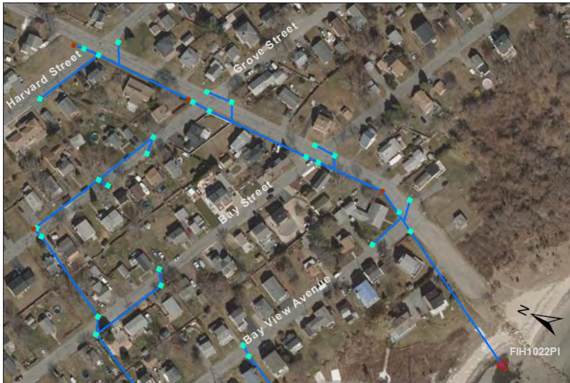
FIH1022PI – Manhattan Ave: no issues found but many of the catchbasins connect to the main drain line without a junction structure.
