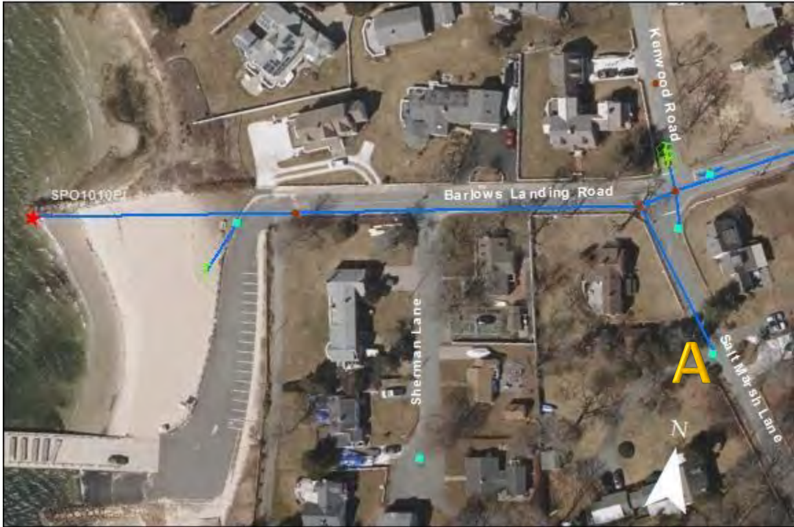
SPO1010PI- Barlows landing Road: No significant issues found. Catchbasin at point A has begun to sink. Preventative maintenance is suggested.
