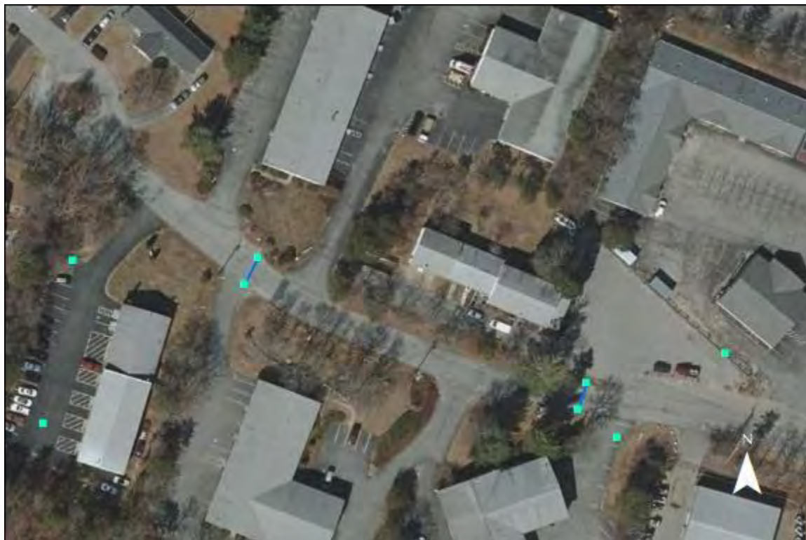
Colonel Drive- No issues found. Catchbasins are infiltration basins.
