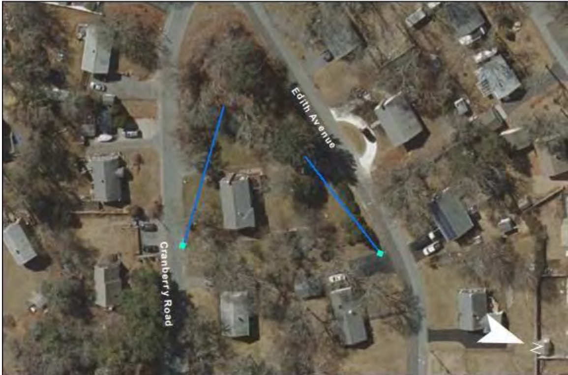
Cranberry Road and Edith Avenue: No issues found. Both pipes travel toward large depression, neither of their destinations could be determined. Further investigation is suggested.
