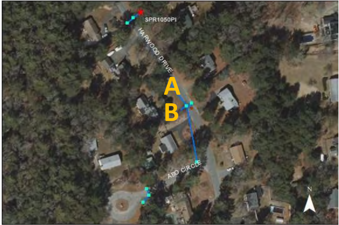
SPR1050PI- Harwood Drive: No significant issues found. At point A and B, two pipes enter the catchbasin. Their origins are unknown. Further investigation is recommended.
