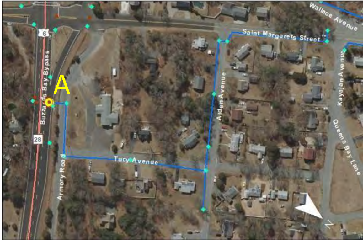
Saint Margaret's Street, Tucey Avenue, and Armory Road: No issues found. At point A the Bourne's stormwater system connects to Massachusetts's stormwater system
