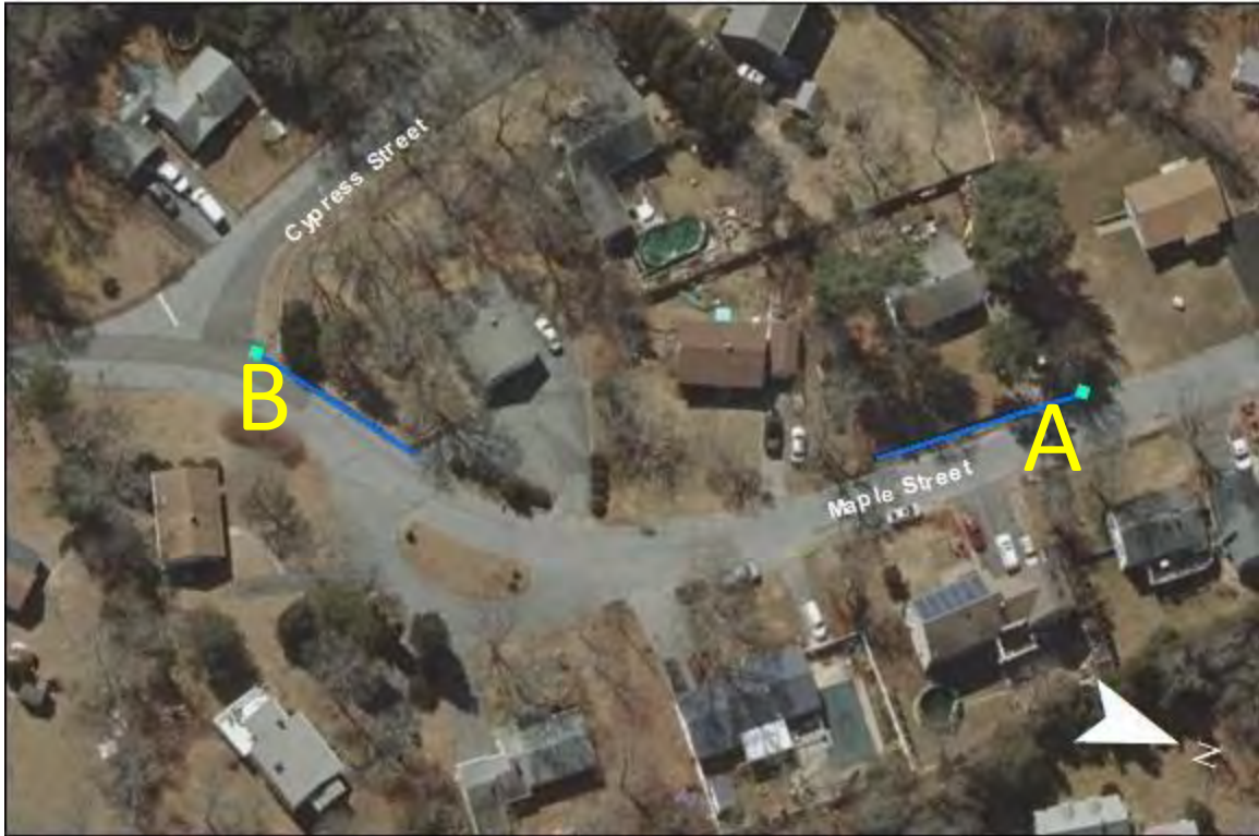
Maple Street: A pipe leaves catchbasin at point A. A pipe enters different catchbasin at point B. Further investigation is suggested to understand if and how these catchbasins connect.
