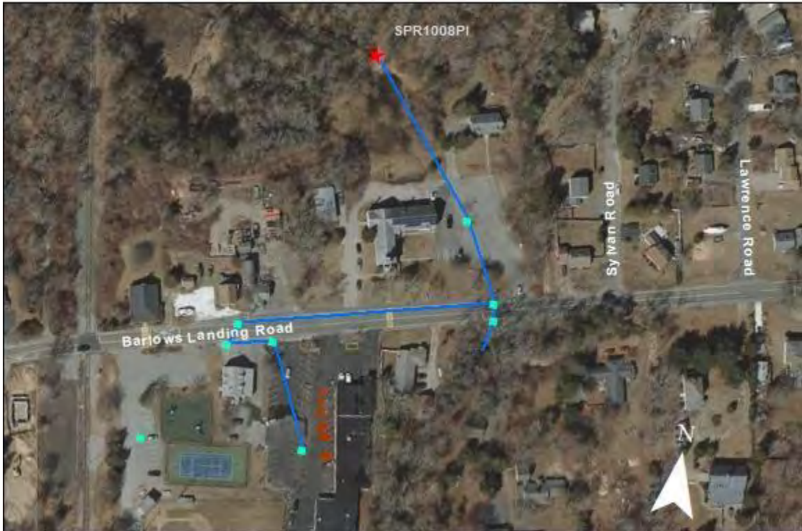
Barlows Landing Road: No significant issues found. Catchbasin at point A is slightly sunken. Preventative maintenance is suggested.
