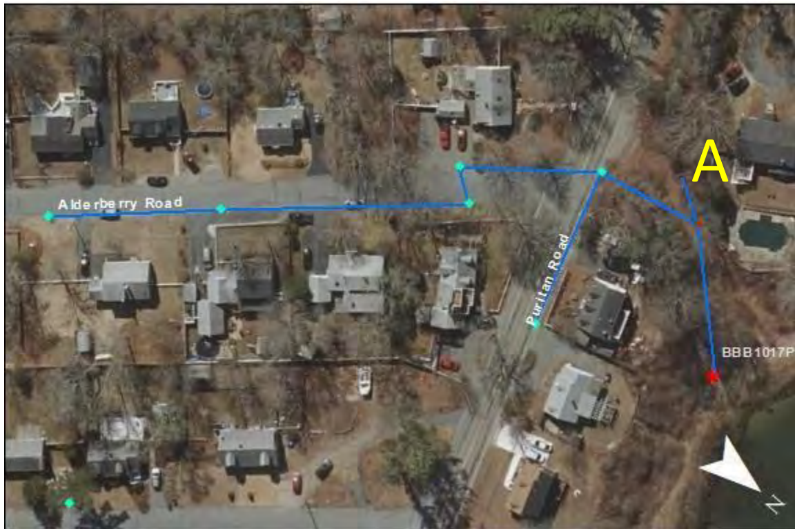
Saint Margaret’s Street, Alden Avenue, Tacy Avenue, and Amory Road: No issues found. At point A Bourne’s stormwater system connects to Massachusetts state’s stormwater system.
