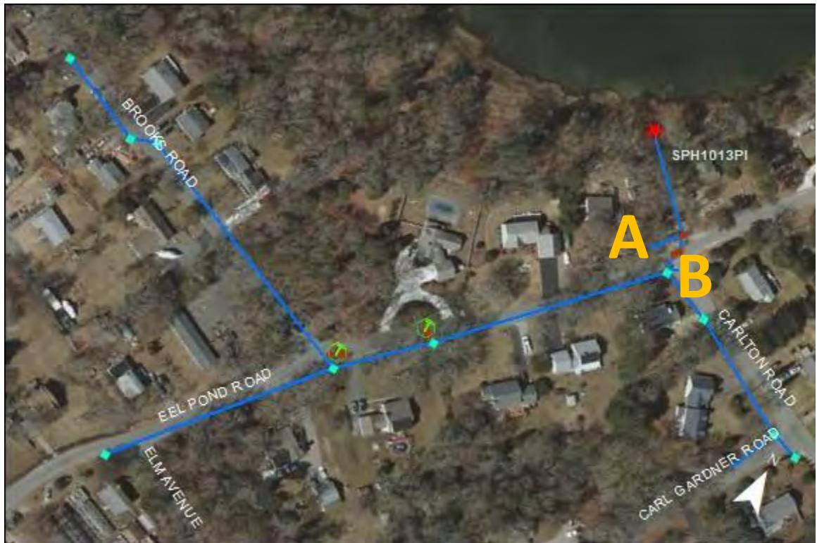
SPR1050PI- Harwood Drive: No significant issues found. At point A and B, two pipes enter the catchbasin. Their origins are unknown. Further investigation is recommended.
