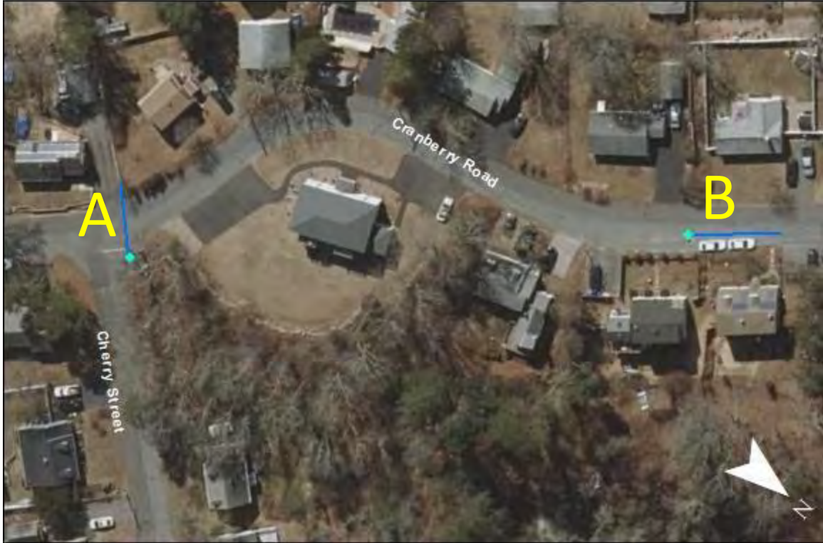
Cherry Street and Cranberry Road: No issues found. At points A and B, pipes were seen leaving the catchbasins, their origin is unknown. Further investigation is recommended.
