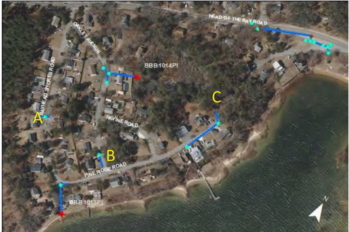
Puritan Road: At point A pipe exists the catchbasin in direction of the cranberry bogs. Kettle Lane: Pipe leaves catchbasin in direction of woods. Destination unknown. Pipe was clogged. Further investigation is needed. Police detail recommended for investigation of structures on Head of the Bay Road.
