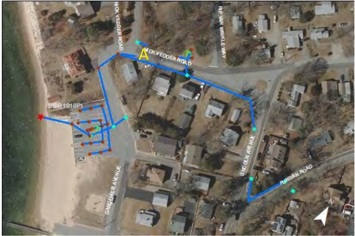
BBB1010PI- Gardenier Avenue: No issues found. This outfall is an overflow for an infiltration chamber under the parking area. The infiltration system appears to be clean and well maintained. There is a pipe entering the manhole at point A. Its origin is unknown. Further investigation is needed.
