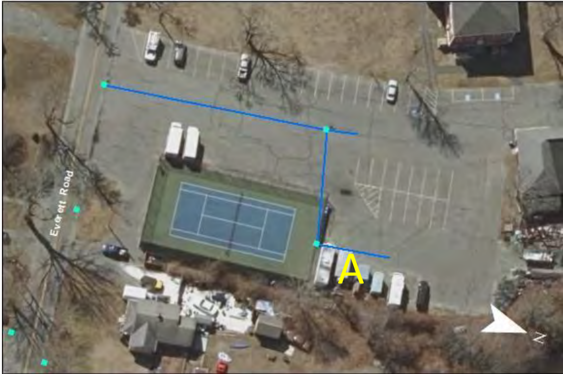
Town Hall parking lot: Pipe at point A is collapsed. An outfall for this catchment has not been able to be identified. Further investigation is suggested.
