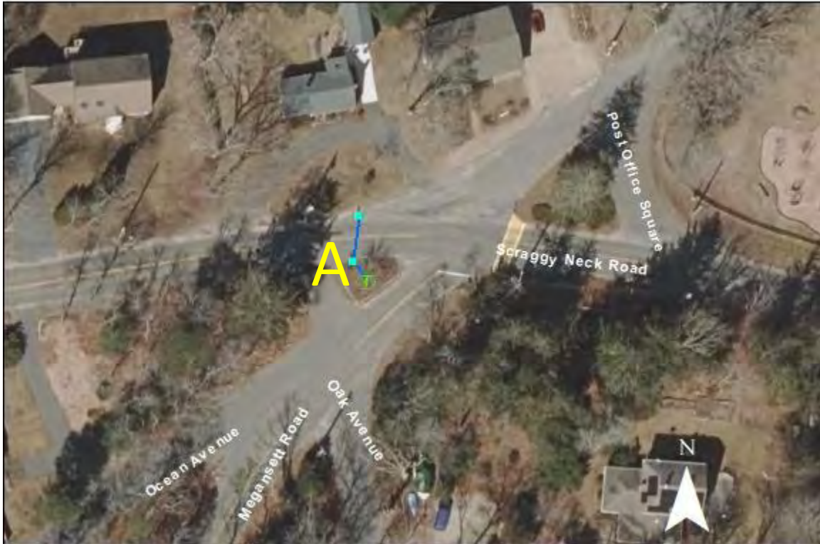
Intersection of Scraggy Neck Road and Ocean Avenue: No significant issues found. The catchbasin at point A is slightly sunken and may need to be repaired.
