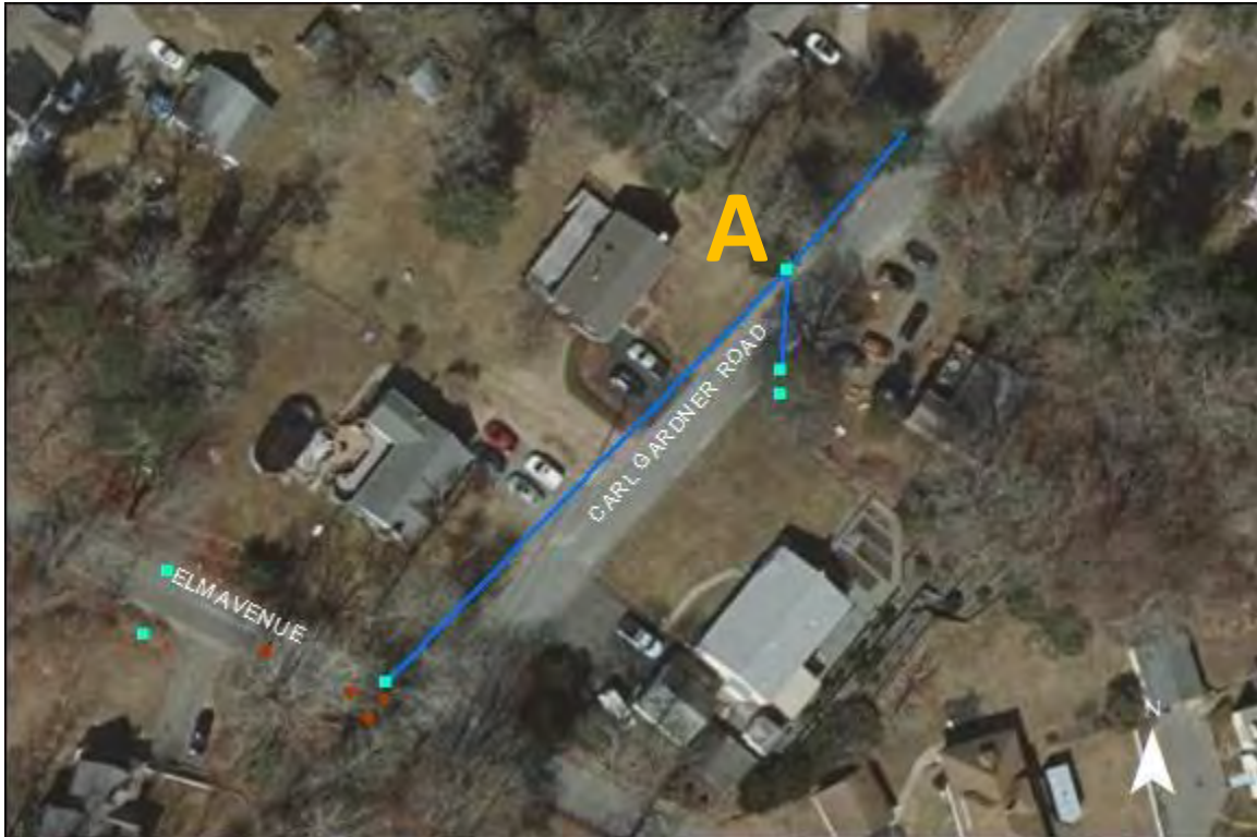
Carl Gardner Road: No significant issues found. Pipe enters catchbasin at point A. Its origin is unknown. Catchment investigation is not complete.
